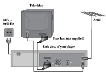
With this connection, if your player is receiving CH ARD and your TV is displaying CH3, when you press the [TV/VCR] button on the remote control, your TV will automatically display the CH ARD. "VCR" will be displayed.
